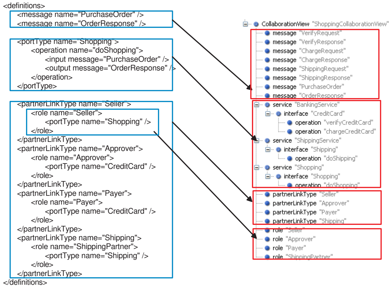
Figure 6. The mapping of the Shopping process descriptions in WSDL to the collaboration view.
