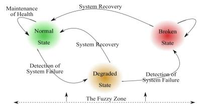
Fig. 4 State diagram of self-healing (taken from [31])
