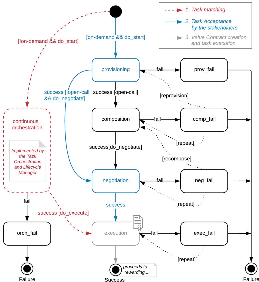
**Figure 2.** Execution model of a WeValue task.
