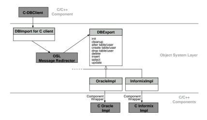
Figure 8. Database Interface With an Object System Layer
