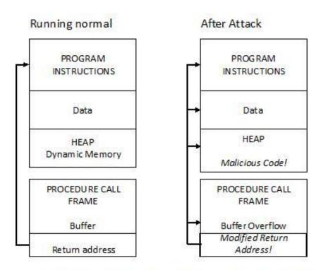
Attacker plants code that overflows buffer and corrupts the return address. Instead of returning to the appropriate calling procedure, the modified return address returns control to malicius code, located elsewhere in process memory.
