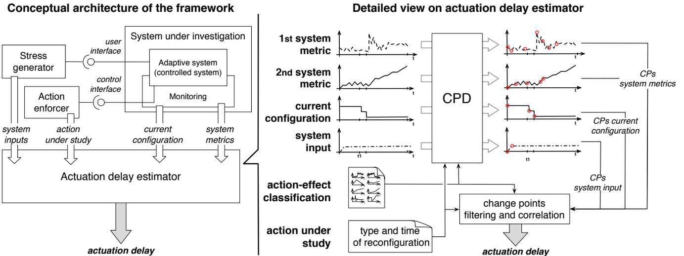
Fig. 4. Conceptual architecture of the delay estimation framework
