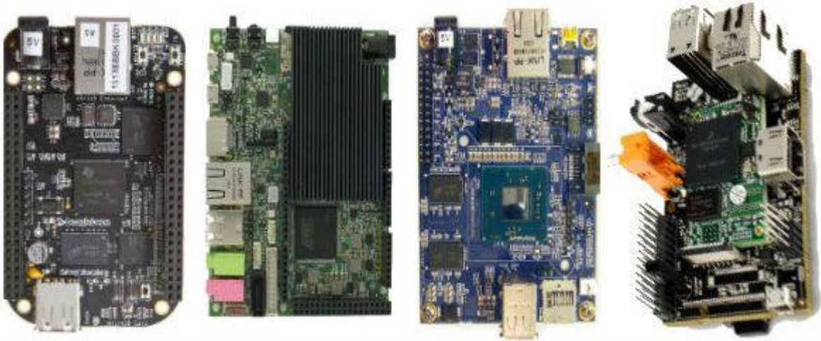
Figure 34: BeagleBone Black, UDOO, MinnowBoard Max and HummingBoard (left to right)
