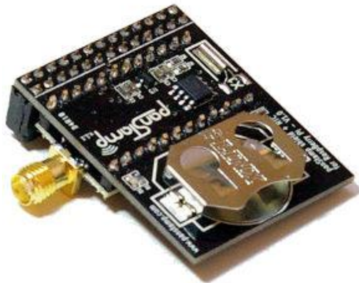
Figure 26: PanStamp shield for the Raspberry Pi [37]
