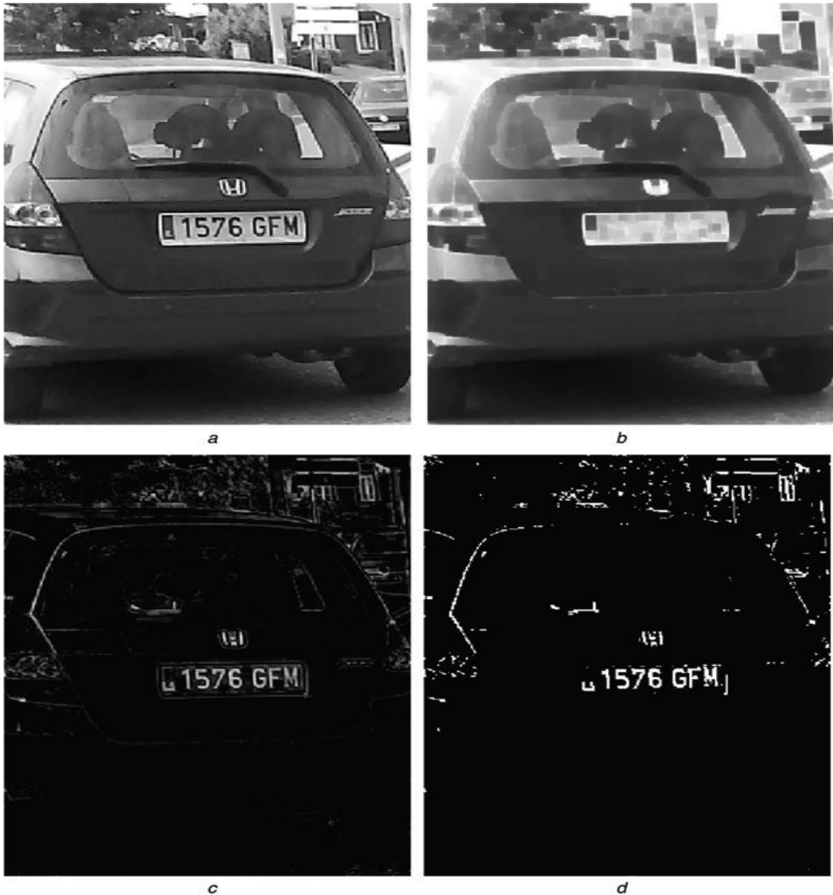
Figure 16: Candidate vehicle (a), morphological closing (b), Top Hat method (c), Otsu method (d) [6]
