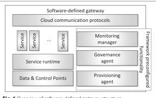
Fig. 6 Overview of software-defined gateway structure
